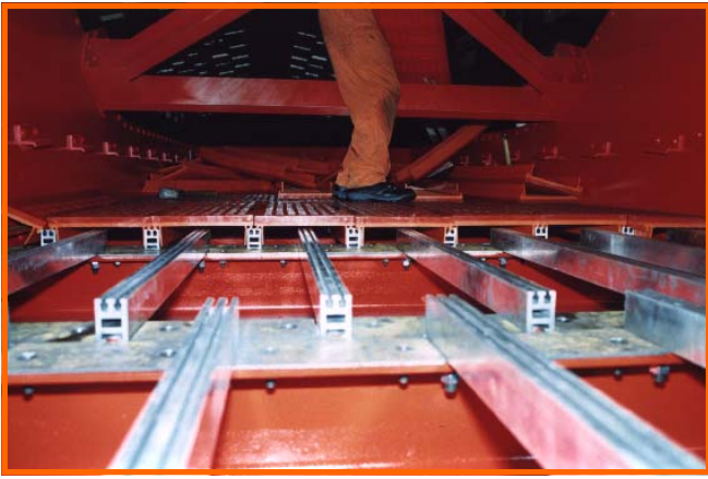
Light alloy SP chanel bolted on the sreen
