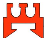
Suitable light alloy channel TYPE II (40 x 25, 5 mm)
