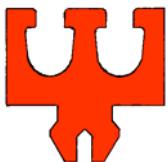
Suitable light alloy channel TYPE I (40 x 25,5 mm)
